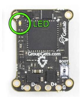
**LED:** When plugged in to power and a Lepton is inserted in the socket LED will flash slowly. When video is being transmitted to the viewing program, LED will flash more rapidly.
